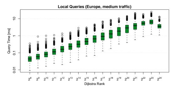
Figure 4: Query time distribution as a function of the Dijkstra-rank of the queries.
