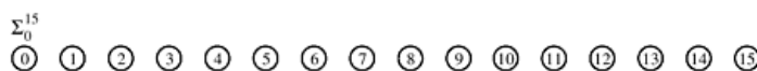
(e) Accumulation of the sum at processing element 0 after the final communication
